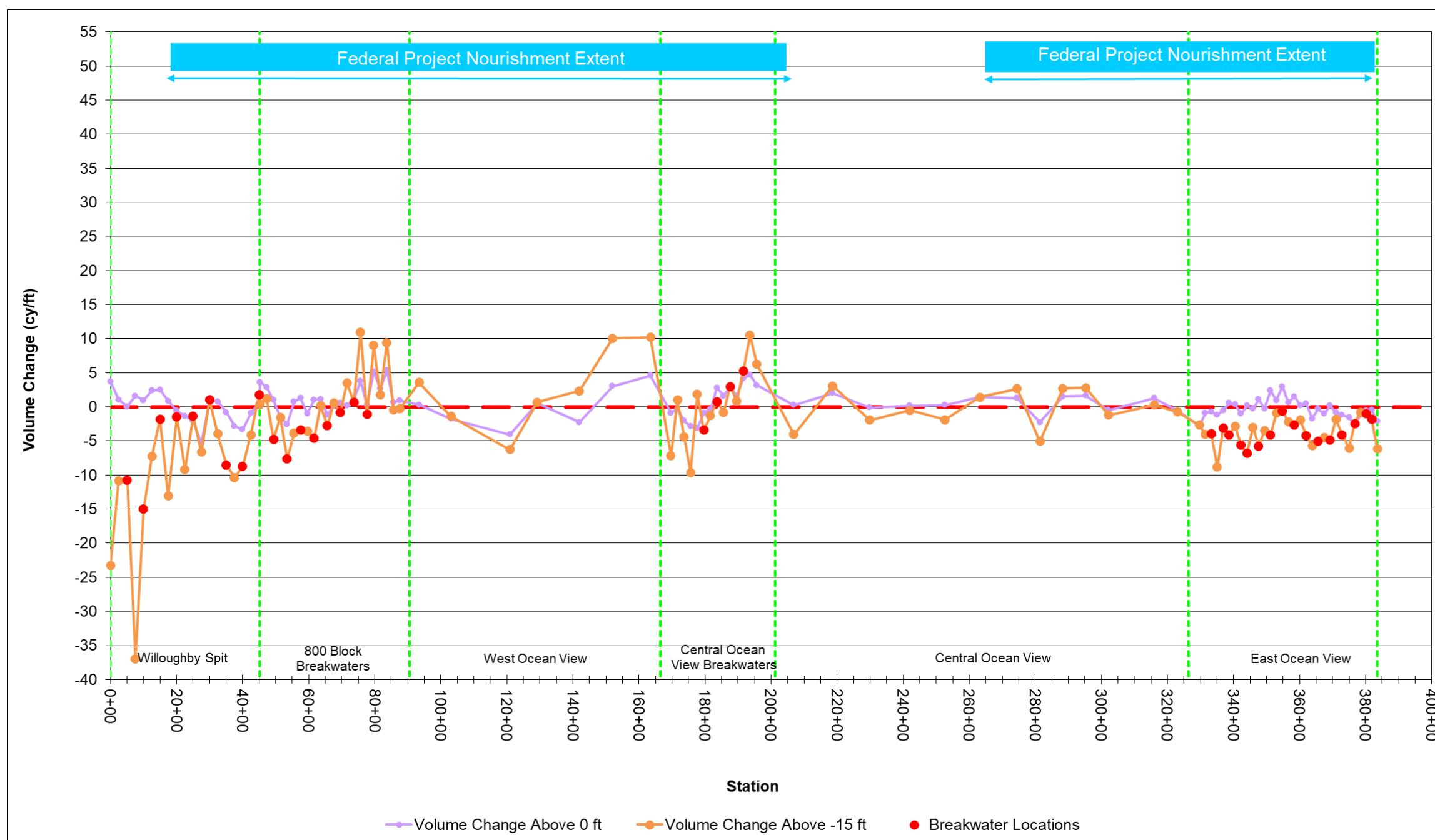
**Figure 5-26: Volume Change above 0 ft NAVD88 and -15 ft NAVD88 (cy/ft) for May 2024 to November 2024 (Note: Positive = Accretion, Negative = Erosion)**
