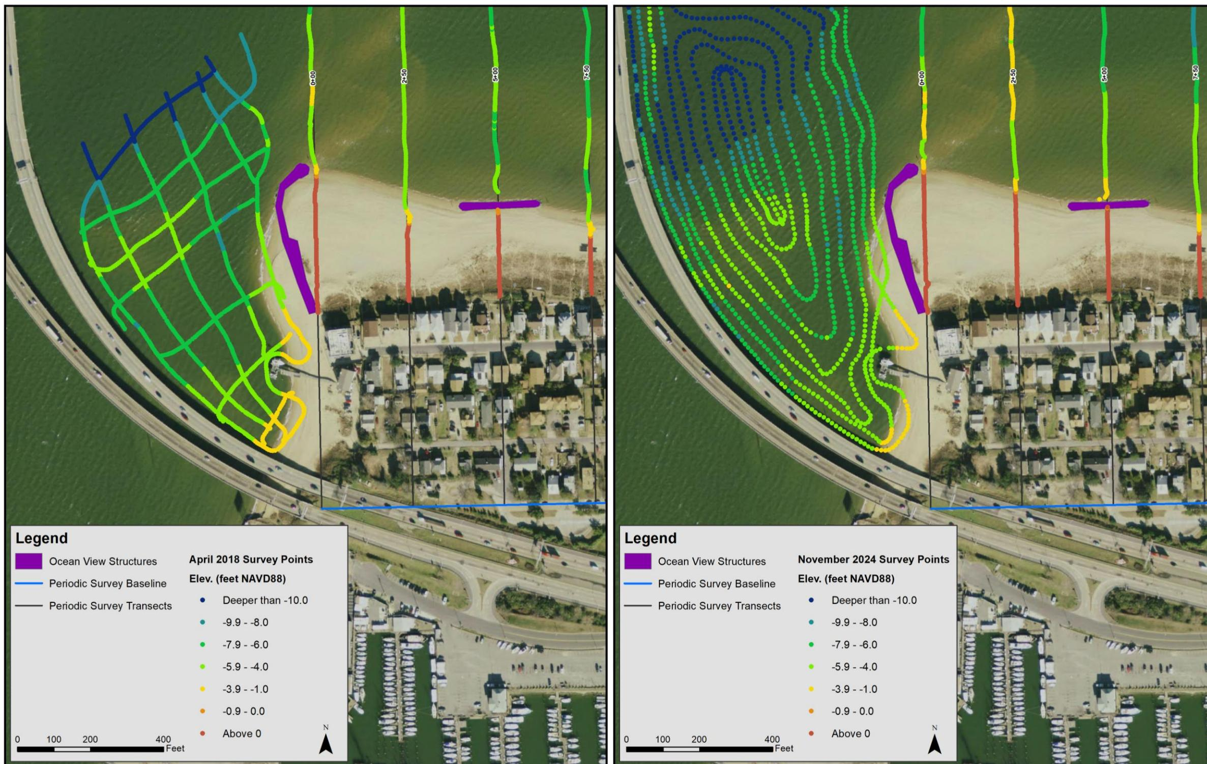
Figure 6-1: Spring 2018 and Fall 2024 Survey Depths West of the Willoughby Spit Terminal Groin
