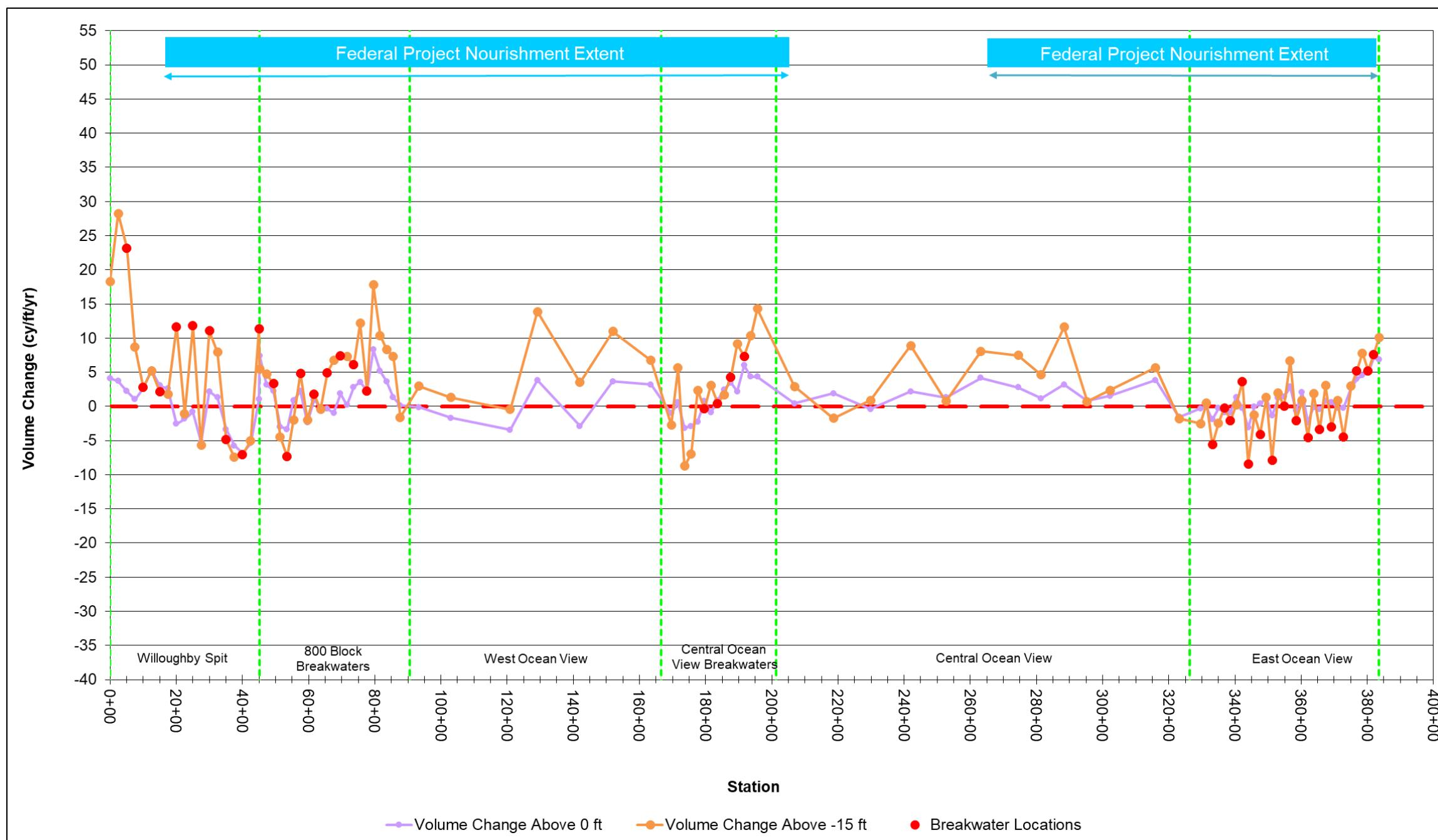
**Figure 5-24: Volume Change Rate Above 0 ft NAVD88 and -15 ft NAVD88 (cy/ft/yr) for November 2023 to November 2024 (Note: Positive = Accretion, Negative = Erosion)**
