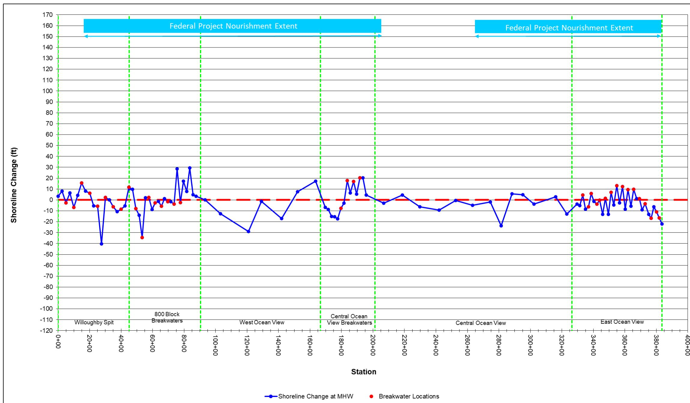
Figure 5-25: Shoreline Change (ft) at Mean High Water (+0.98 ft NAVD88) for May 2024 to November 2024 (Note: Positive = Accretion, Negative = Erosion)
