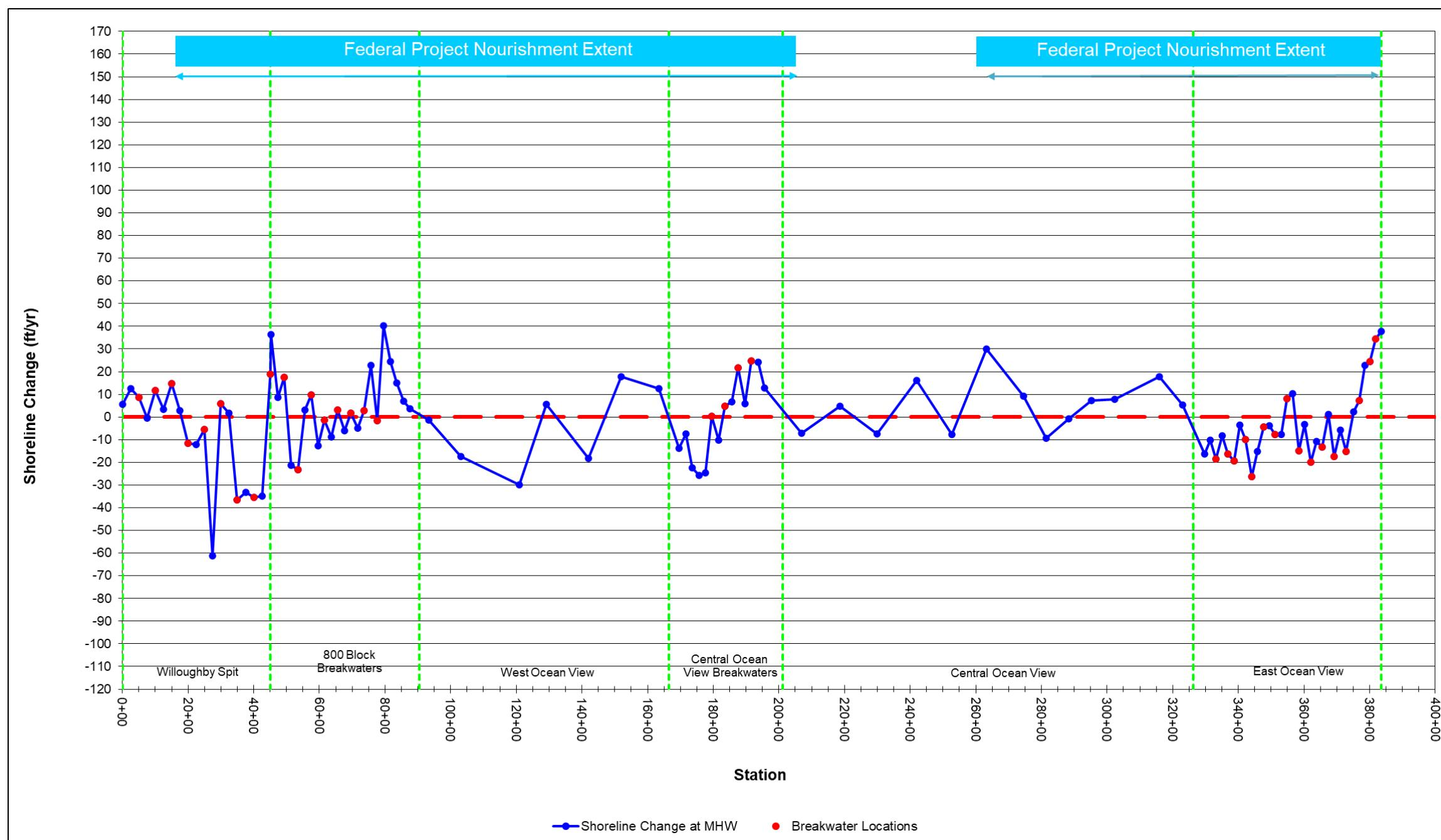
Figure 5-23: Shoreline Change Rate (ft/yr) at Mean High Water (+0.98 ft NAVD88) for November 2023 to November 2024 (Note: Positive = Accretion, Negative = Erosion)
