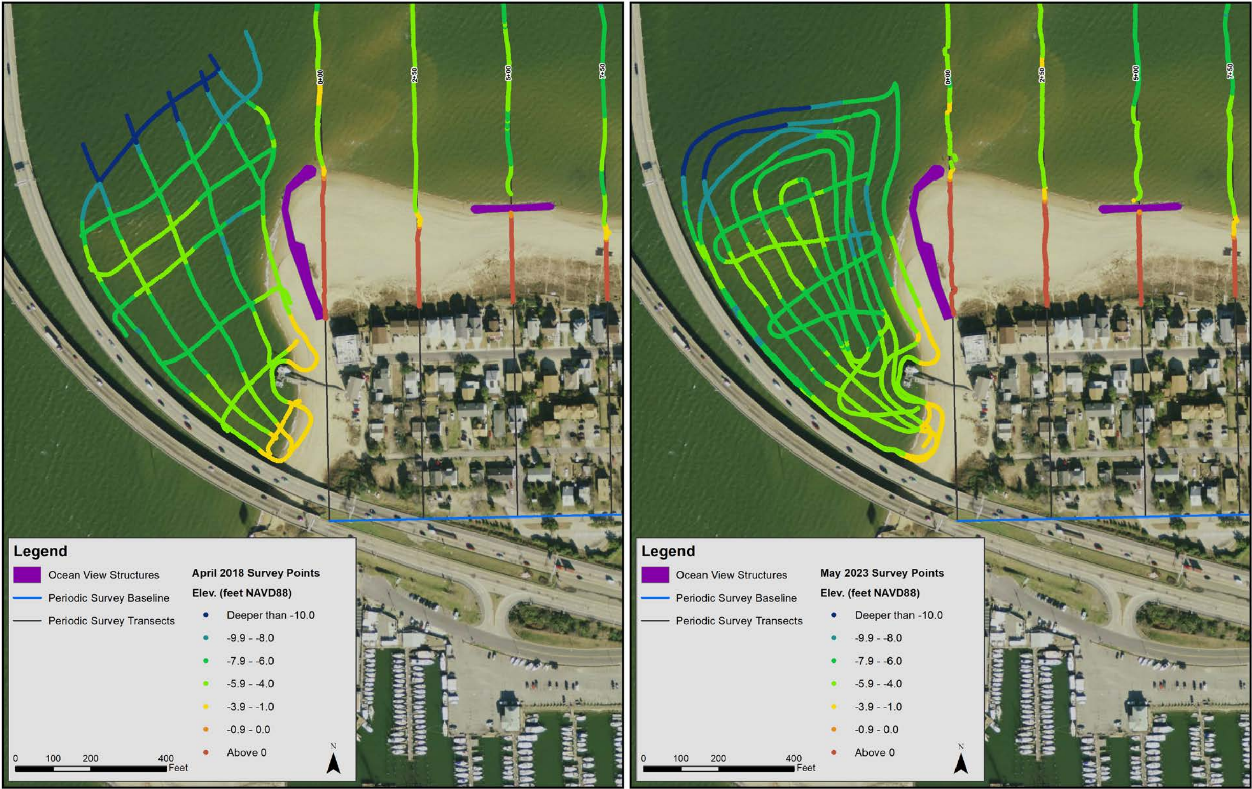
Figure 6-1: Spring 2018 and Spring 2023 Survey Depths West of the Willoughby Spit Terminal Groin
